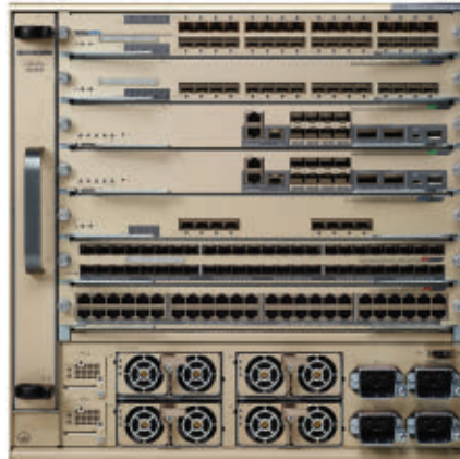
The Cisco 6807 Ethernet switch is used in both shipboard and fixed-base installations to provide a high-speed network core.
